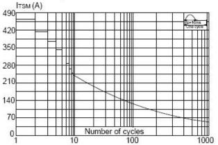
FIG.5: Non-repetitive surge peak on-state current for a sinusoidal pulse with width tp<10ms, and corresponging value of I²t (dI/dt < 50A/μs)
